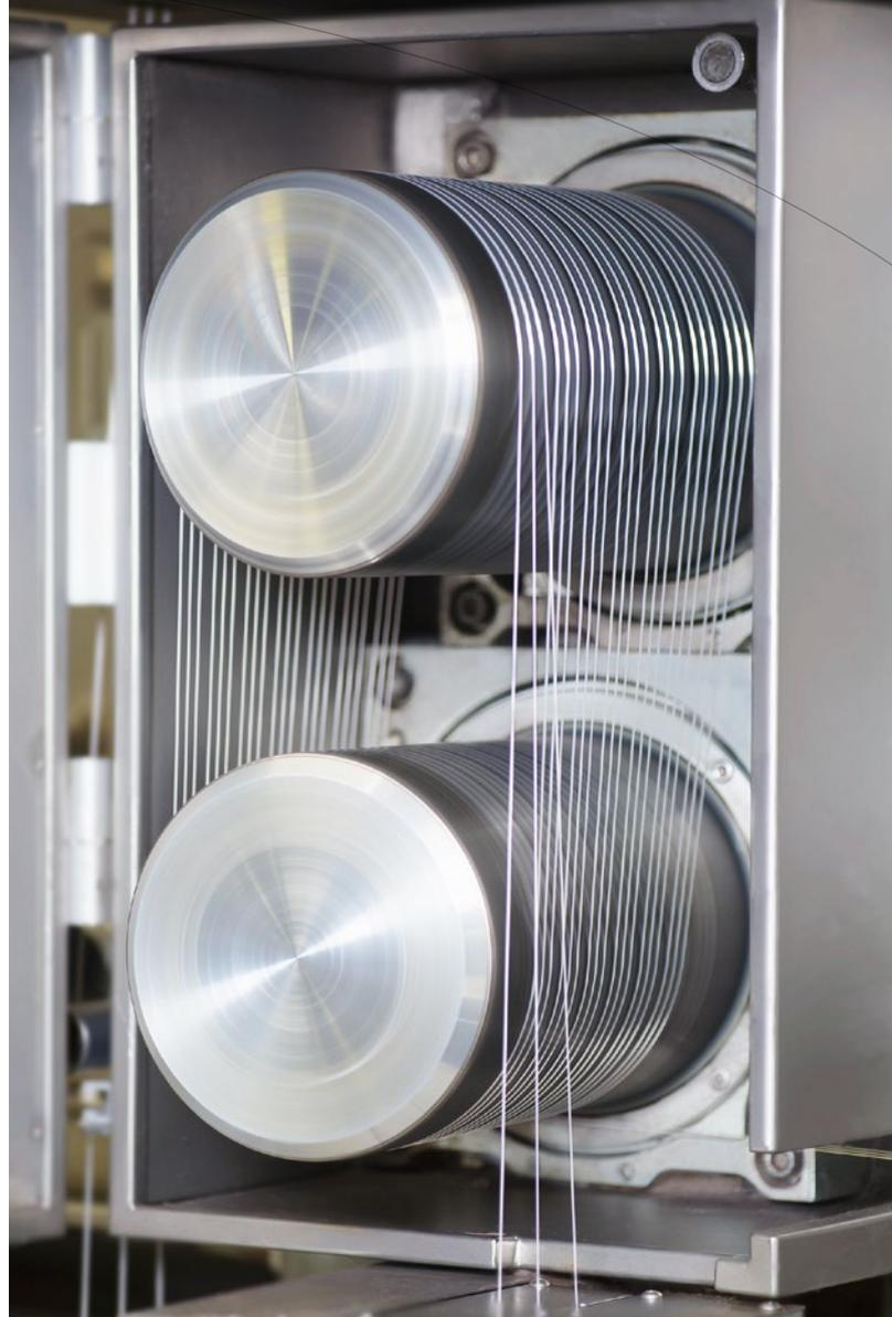
Inductive heating in synthetic fiber production (picture: © Oerlikon Neumag)
